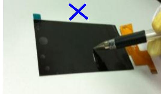
Please don't operate with sharp stick such as pens 请不要用尖锐的物体来操作，例如用笔尖
